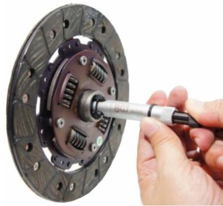
Install the clutch disc with clutch pressure plate.
