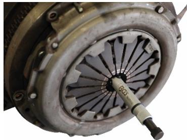
Press the clutch aligning tool with clutch disc toward the engine and evenly tighten the mounting screws of clutch pressure plate succession. Tighten the screws at the end with the specified torque.
