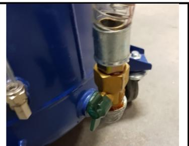
Close the shut-off valve on the suction hose (2)
