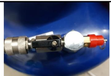
Slowly open the shut-off valve on the tank base. In doing so, make sure that the pipe elbow of the emptying hose remains in the waste oil tank.
