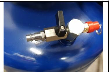
Close the shut-off valve under the measuring cylinder.
