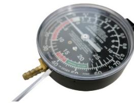
Take a slot screwdriver and turn the adjusting screw in the direction in which the pointer must be re-adjusted. In the shown example, the adjustment screw must be turned clockwise.
