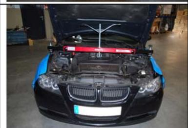
Adjust the angle of engine support and fix the setting with the lateral screws.
