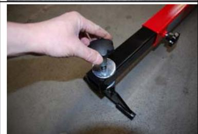
Insert the holding screw into the centre hole of the middle piece and tighten the large wing nut on the holding screw a few turns.
