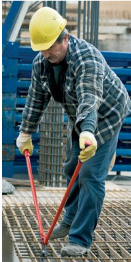
The special shape of the mesh cutter head, 71 82 950, enables it to cut structural steel that is lying down flat
