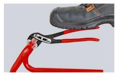
Self-locking on pipes and nuts: no slipping on the workpiece; the complete actuating force can be used to turn the workpieces; not having to squeeze the pilers handles reduces the required effort
