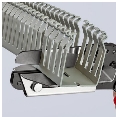
Blade length 110 mm for cutting wide cable ducts
