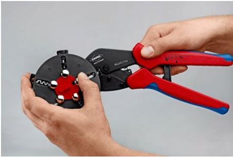
Changing the crimping dies: unlock the magazine position, take out the set of dies which the pliers have been pushed on
